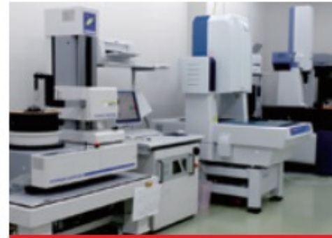
Roundness measuring machine (Tokyo Seimitsu)
