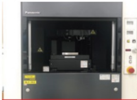
Ultrahigh accurate 3-D profilometer (Panasonic)
