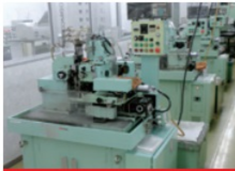
Centerless grinding machine (Imahashi)
