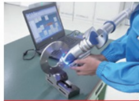
FARO portable 3D measuring instrument (FARO)
