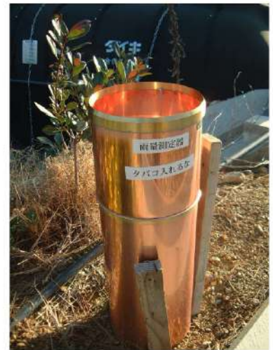
Collecting micro climate data on site by measuring the temperature, humidity, earth temperature and rainfall in order to make use of it.
